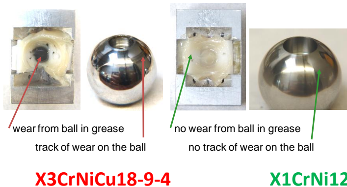
Figure 16: Friction behavior of austenitic steel X3CrNiCu18-9-4 and ferritic steel X1CrNi12 in ball-prism-tribometer versus greased POM after a friction path of 1700 mm
