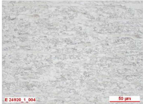
Figure 5: Microstructure of the X1CrNi12 stainless steel in as-rolled condition
