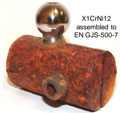
Figure 13: Corrosion of a pin made of X1CrNi12 after 10 cycles in a VDA alternating climate test, assembled in GGG40
