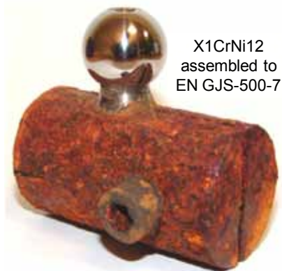
Figure 7: Corrosion of a pin made of X1CrNi12 after 10 cycles in a VDA alternating climate test, assembled in GGG40
