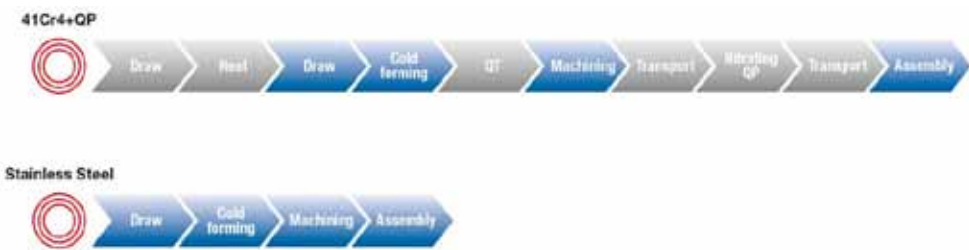
Figure 1: Elimination of process steps by using stainless steels as an alternative to nitrided quenched and tempered steels
