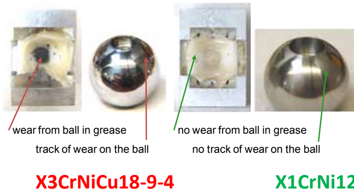
Figure 9: Friction behavior of austenitic steel X3CrNiCu18-9-4 and ferritic steel X1CrNi12 in ball-prism-tribometer versus greased POM after a friction path of 1700 mm
