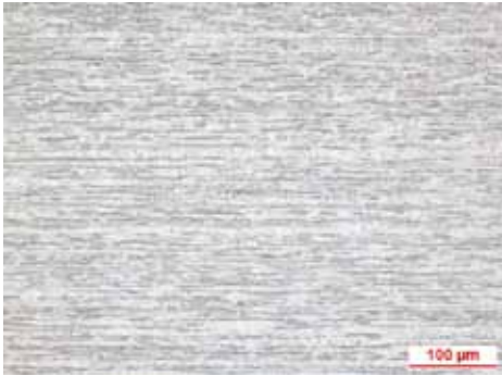
Figure 2: Microstructure of the X1CrNi12 stainless steel in as-rolled condition
